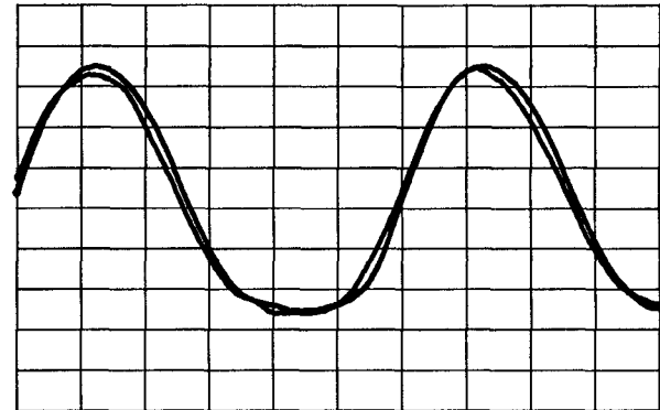
Figure 7: Saturation at drains 4 and 5 of microstrip TWA; 3 GHz, 7 dBm input power
